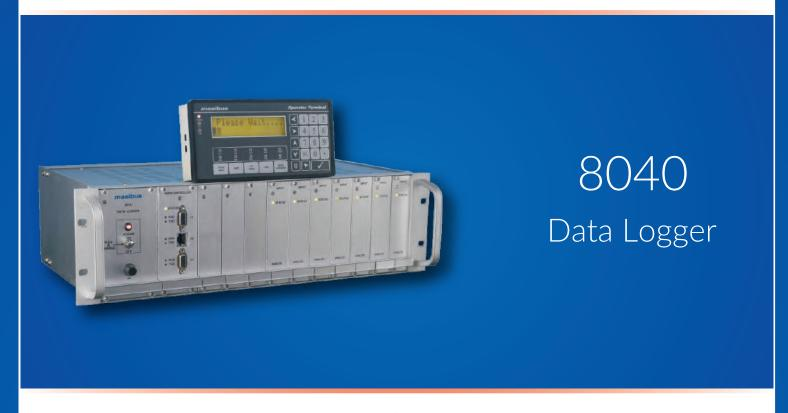
Masibus Datalogger Model 8040 is a high performance Data Acquisition/Data logging Device, designed to work as a standalone unit or with PC Interface. Model 8040 is available in 19" sub-rack with 10 I/O slots, the architecture supports a max of 8 universal Analog input modules and max of 2 Digital output modules (1 DO only possible in case of Ethernet or USB o/p in Main Controller), Power Supply and Main Controller Module.
